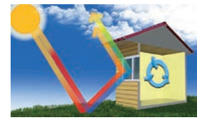
Low-E reduces solar heat gain by diffusing radiation coming from the sun.
